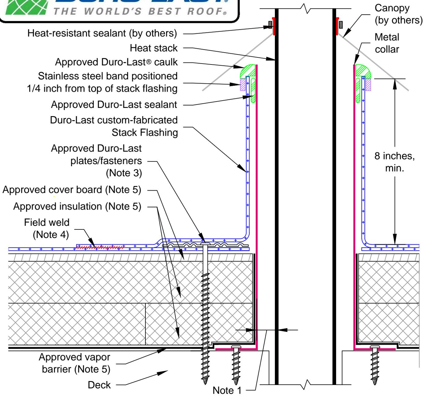
Note 1: This detail is required around heat stacks that exceed 120° F, including all insulated chimney stacks. A minimum of 1-inch air space is required between the metal collar and heat stack. The canopy must be positioned to allow adequate air flow above the termination.
