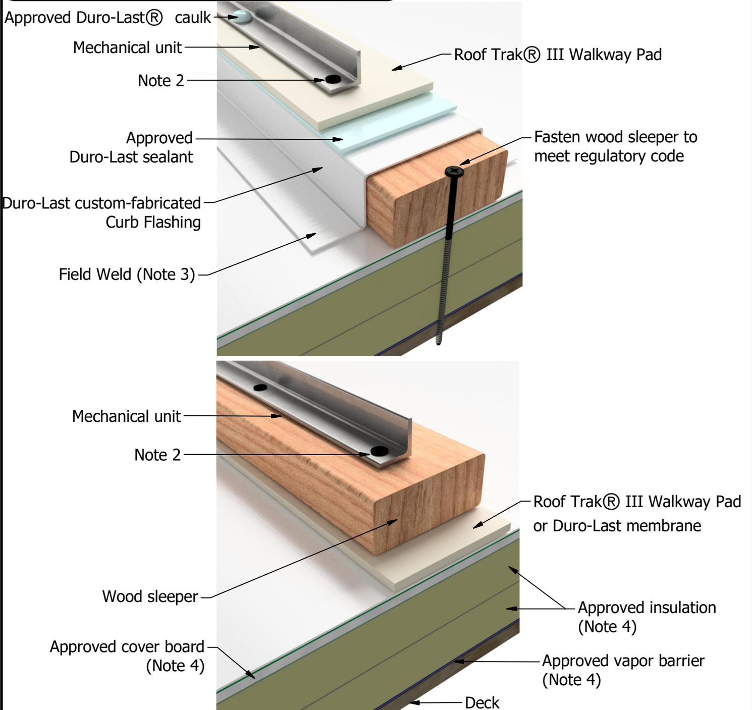
Note 1: If the mechanical units are of a size that they will crush the insulation, then the insulation below the sleeper must be replaced by wood blocking.
