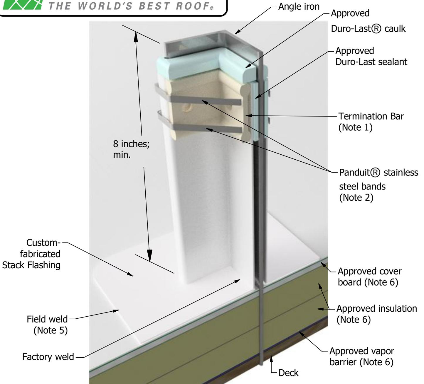
Note 1: Cut Termination Bar slightly larger than side of angle iron to allow for compression of Termination Bar by Panduit bands.
