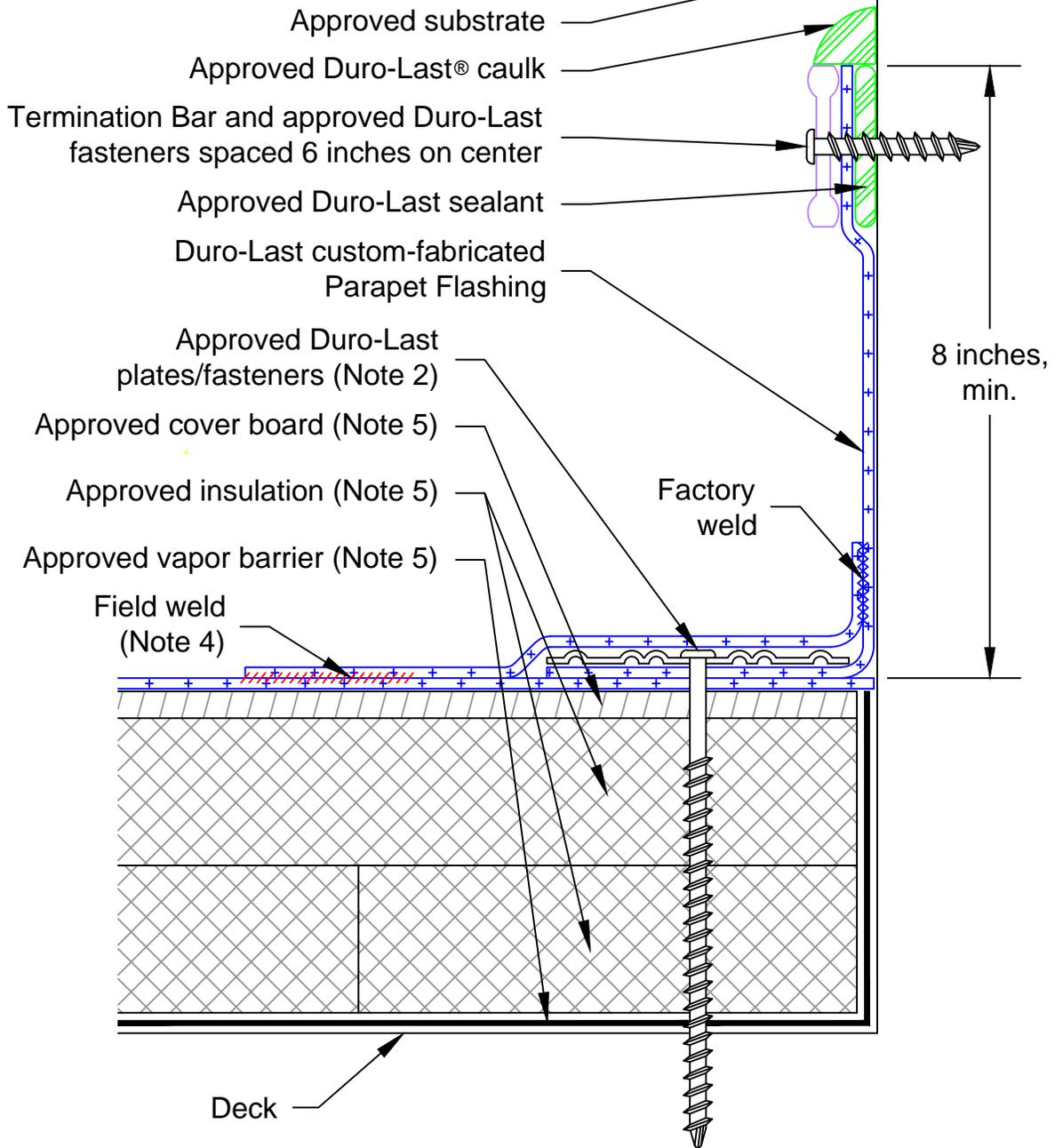
Note 1: 1-3/4 or 4-inch Fascia Bar and Cover (cover optional) may be used in place of Termination Bar.
