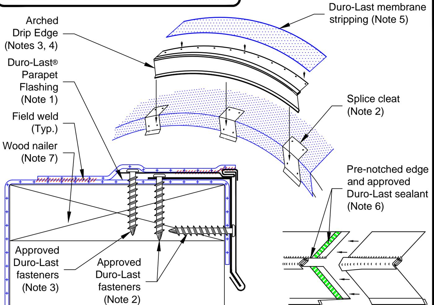
Note 1: Install Duro-Last Parapet Flashing as per Detail Drawing 6010.
