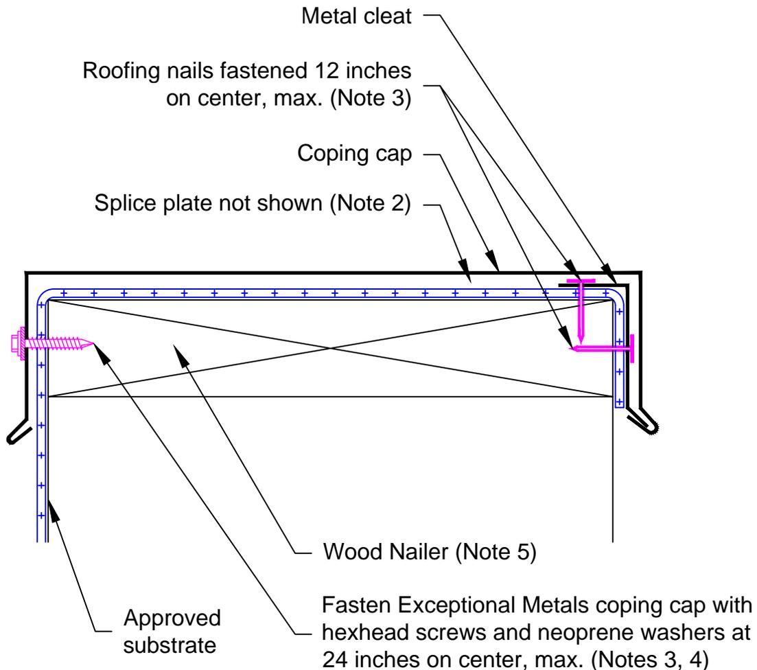
Note 1: All coping cap joints must utilize a 6-inch concealed splice plate.
