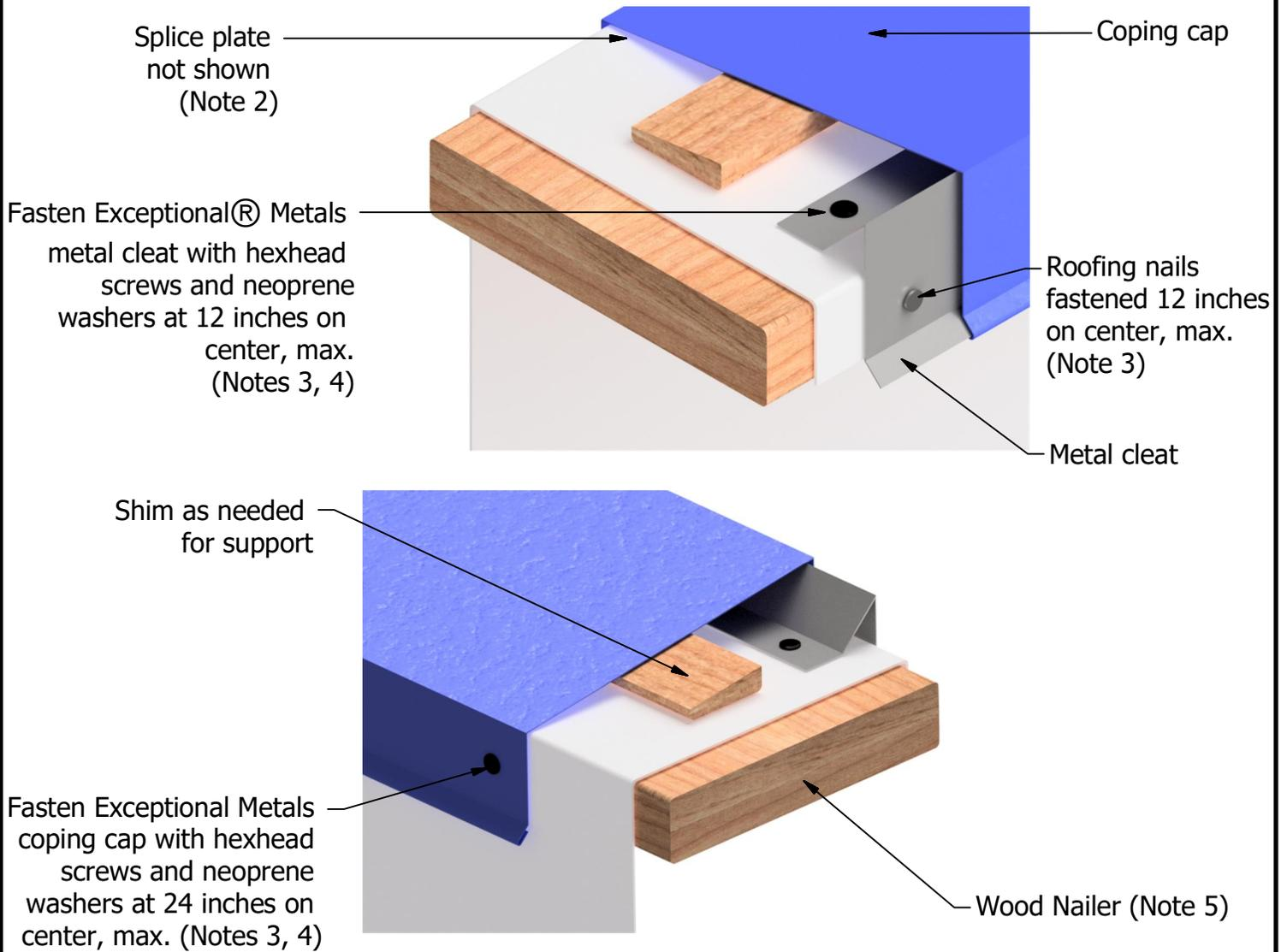
Note 1: All coping cap joints must utilize a 6-inch concealed splice plate.
