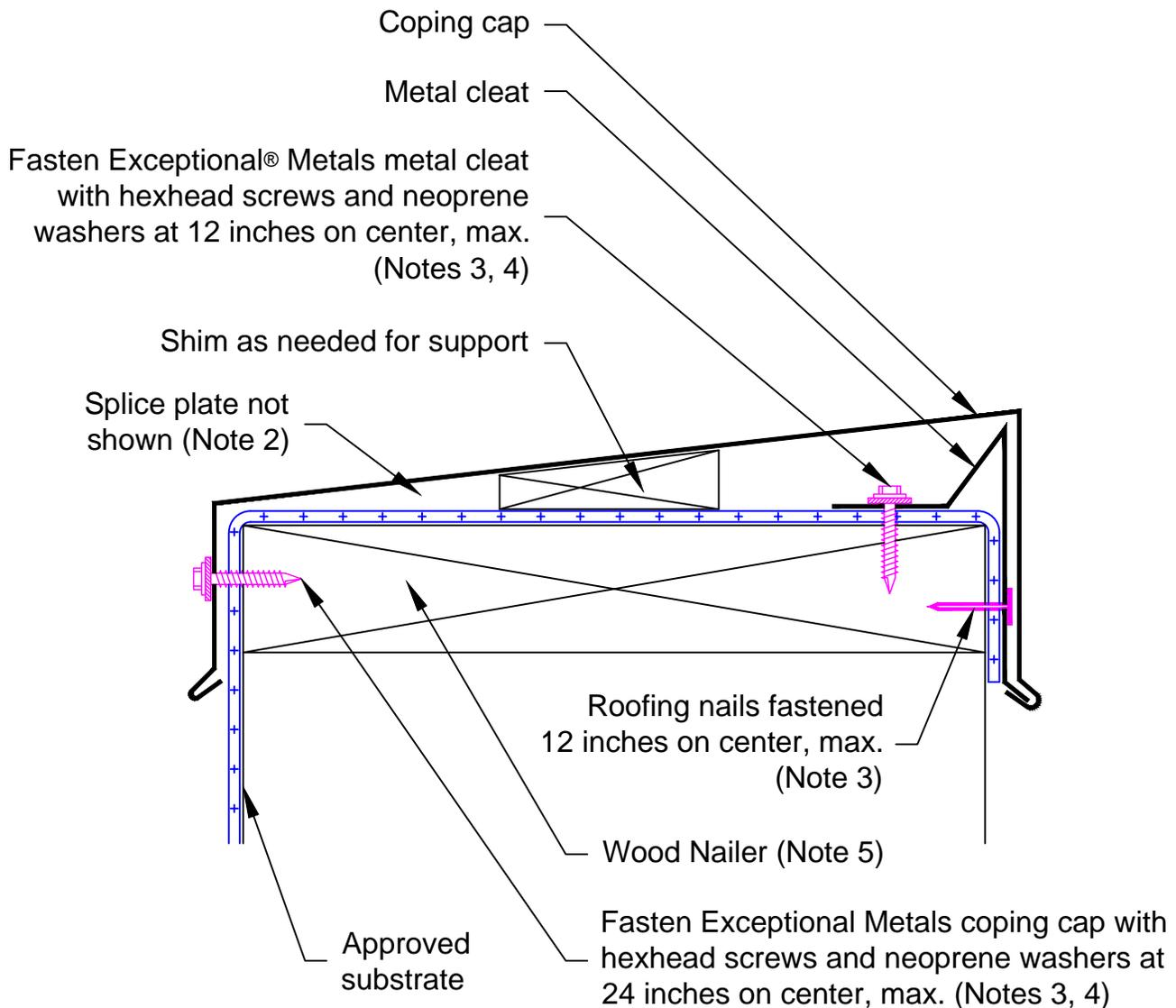
Note 1: All coping cap joints must utilize a 6-inch concealed splice plate.
