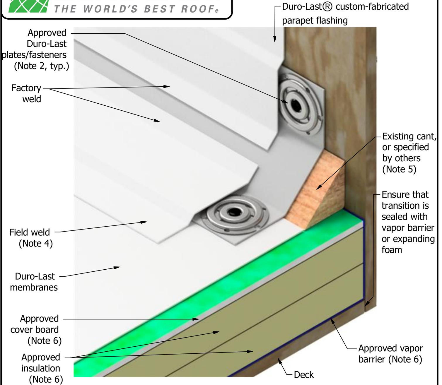
Note 1: Minimum termination height for parapet wall flashing is 8 inches above finished deck. Refer to Detail Drawing 6020.
