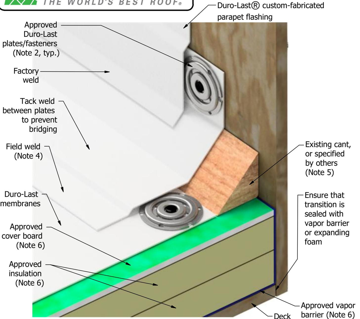
Note 1: Minimum termination height for parapet wall flashing is 8 inches above finished deck. Refer to Detail Drawing 6020.
