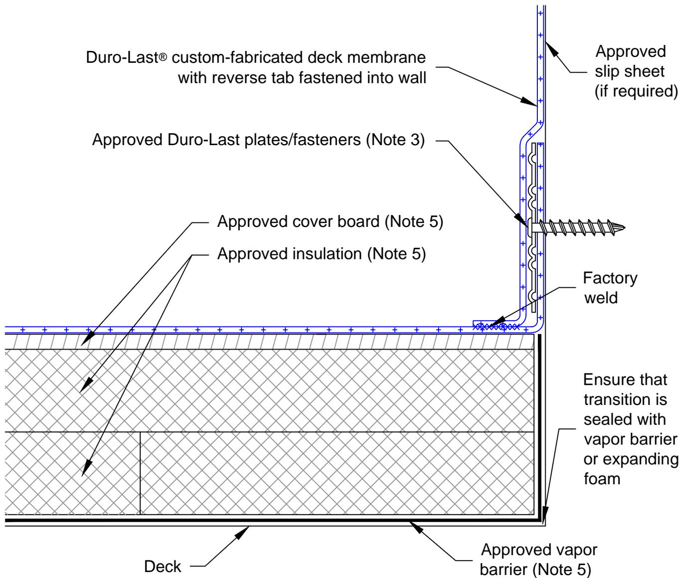
Note 1: It is not recommended to exceed 18 inches in height when using deck sheet reverse tabs to flash walls.
