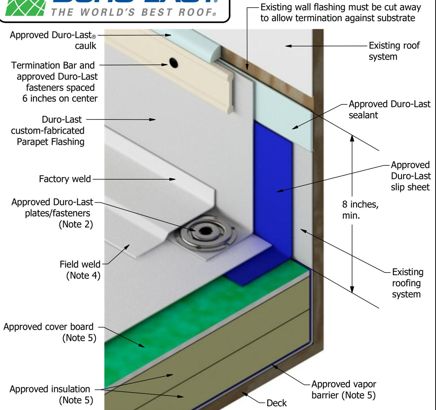
Note 1: 1-3/4 or 4-inch Fascia Bar and Cover (cover optional) may be used in place of Termination Bar.
