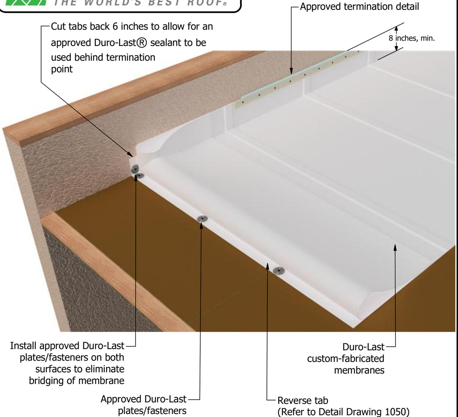
Note 1: This detail cannot be used when fastening tab spacing exceeds 60 inches.
