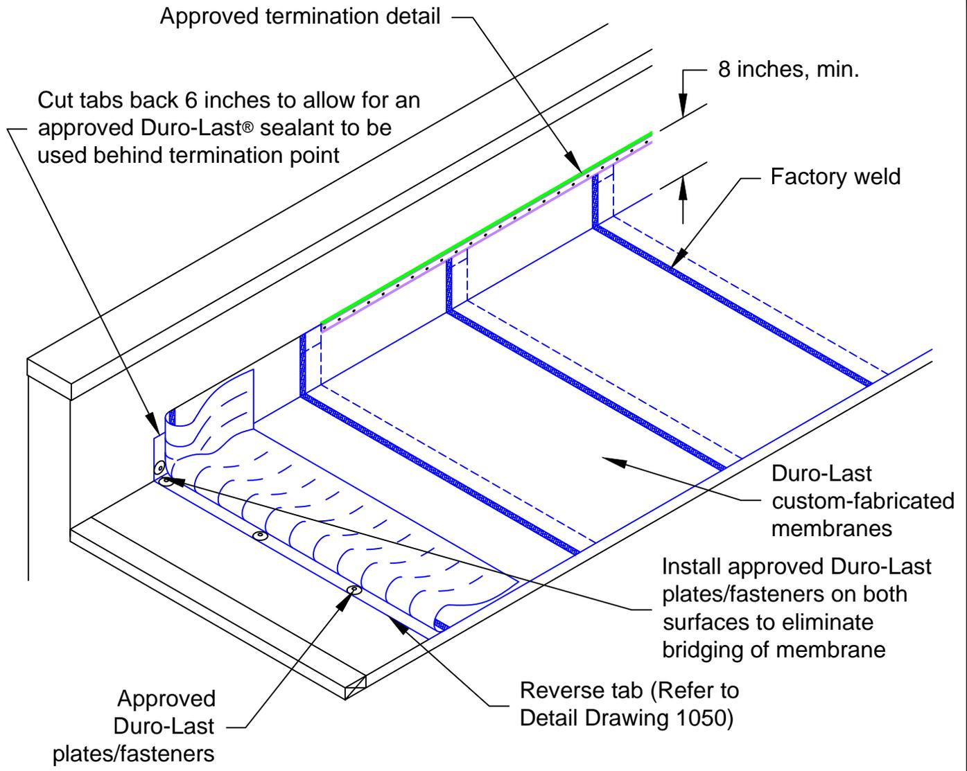
Note 1: This detail cannot be used when fastening tab spacing exceeds 60 inches.
