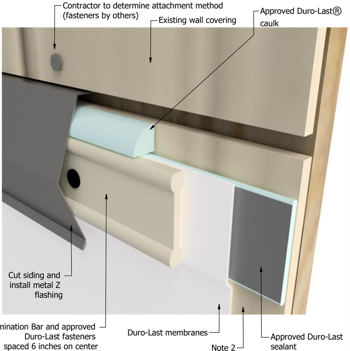
Note 1: Minimum termination height for parapet wall flashing is 8 inches above finished deck. Refer to Detail Drawing 6020.
