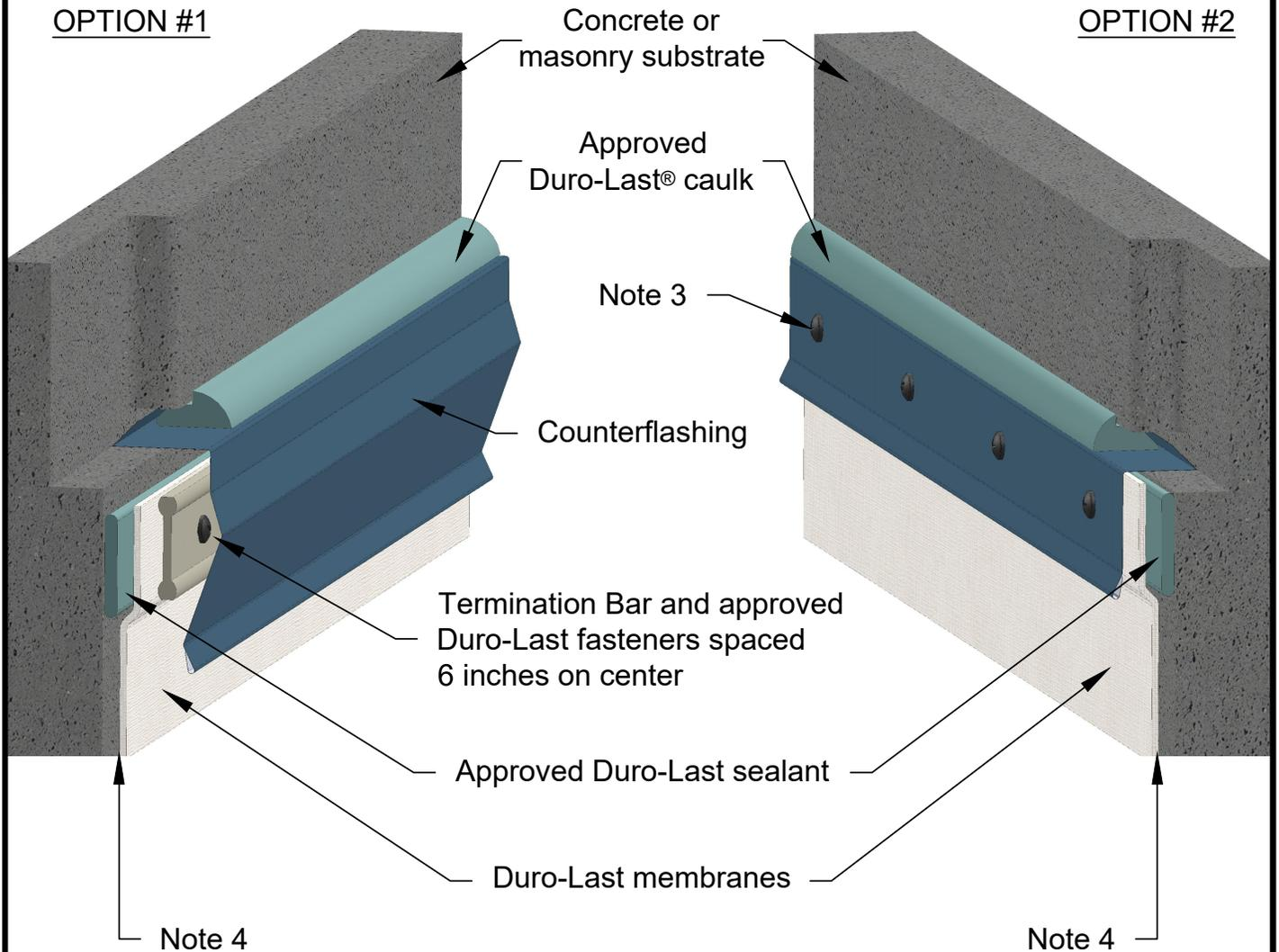
**Note 1: This detail is only applicable with concrete or masonry walls.**
