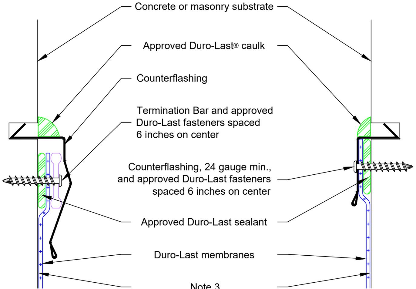
**Note 1: This detail is only applicable with concrete or masonry walls.**
