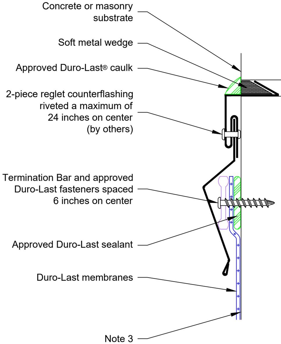
**Note 1: This detail is only applicable with concrete or masonry walls.**
