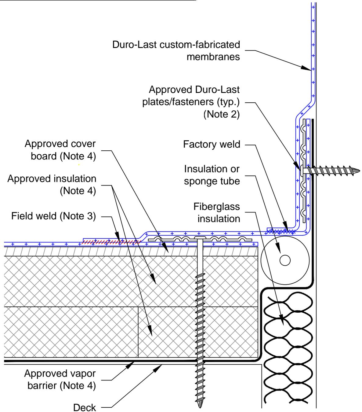
Note 1: This detail is required when there are gaps between deck and parapet wall.
