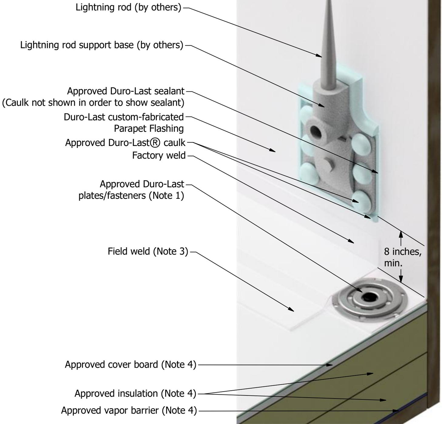
Note 1: Membrane fastening at deck-to-wall transitions and walls shall be same as per respective zones that area is located within (field, perimeter, corner).
