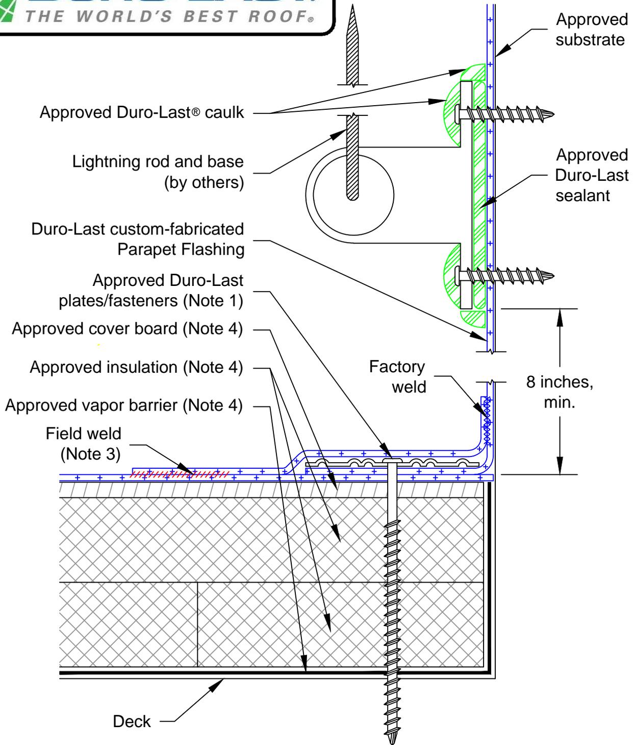
Note 1: Membrane fastening at deck-to-wall transitions and walls shall be same as per respective zones that area is located within (field, perimeter, corner).
