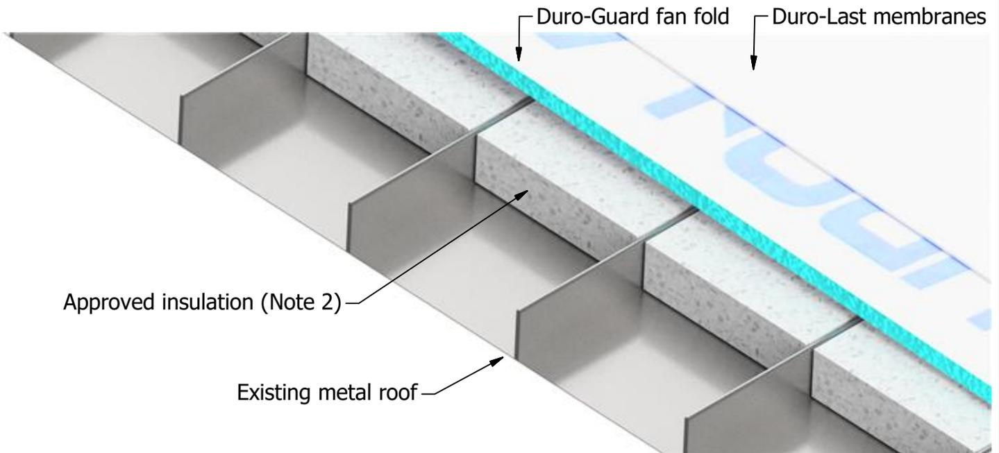
Note 1: Duro-Guard fan fold may be used over flute filler on a metal roof if span between flute filler and flute does not exceed 1/4 inch.
