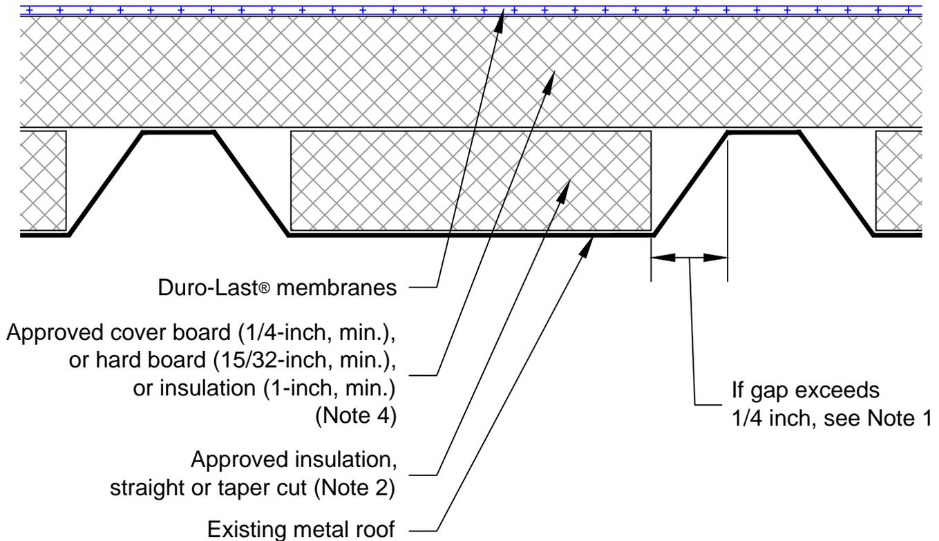
Note 1: Gaps must not exceed spanability of insulation, cover board or hard board. See Product Data Sheet for spanability of each specific product used.
