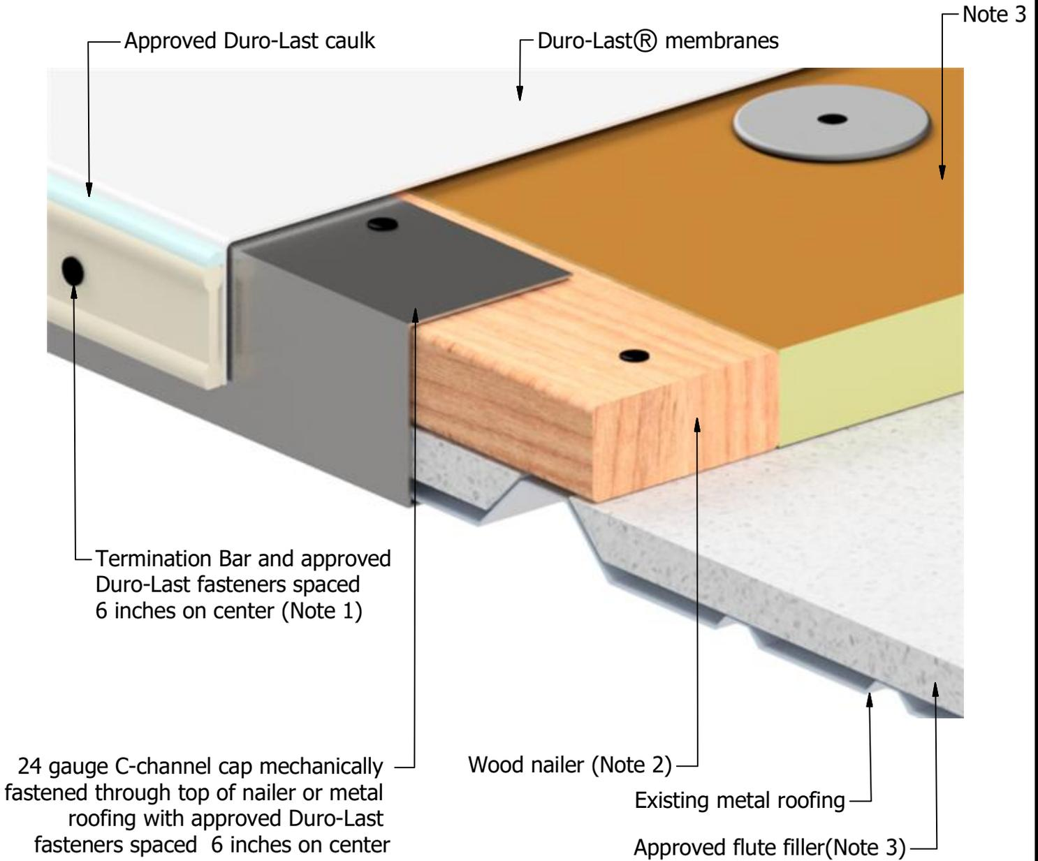
Note 1: Approved edge details may be used in place of Termination Bar.
