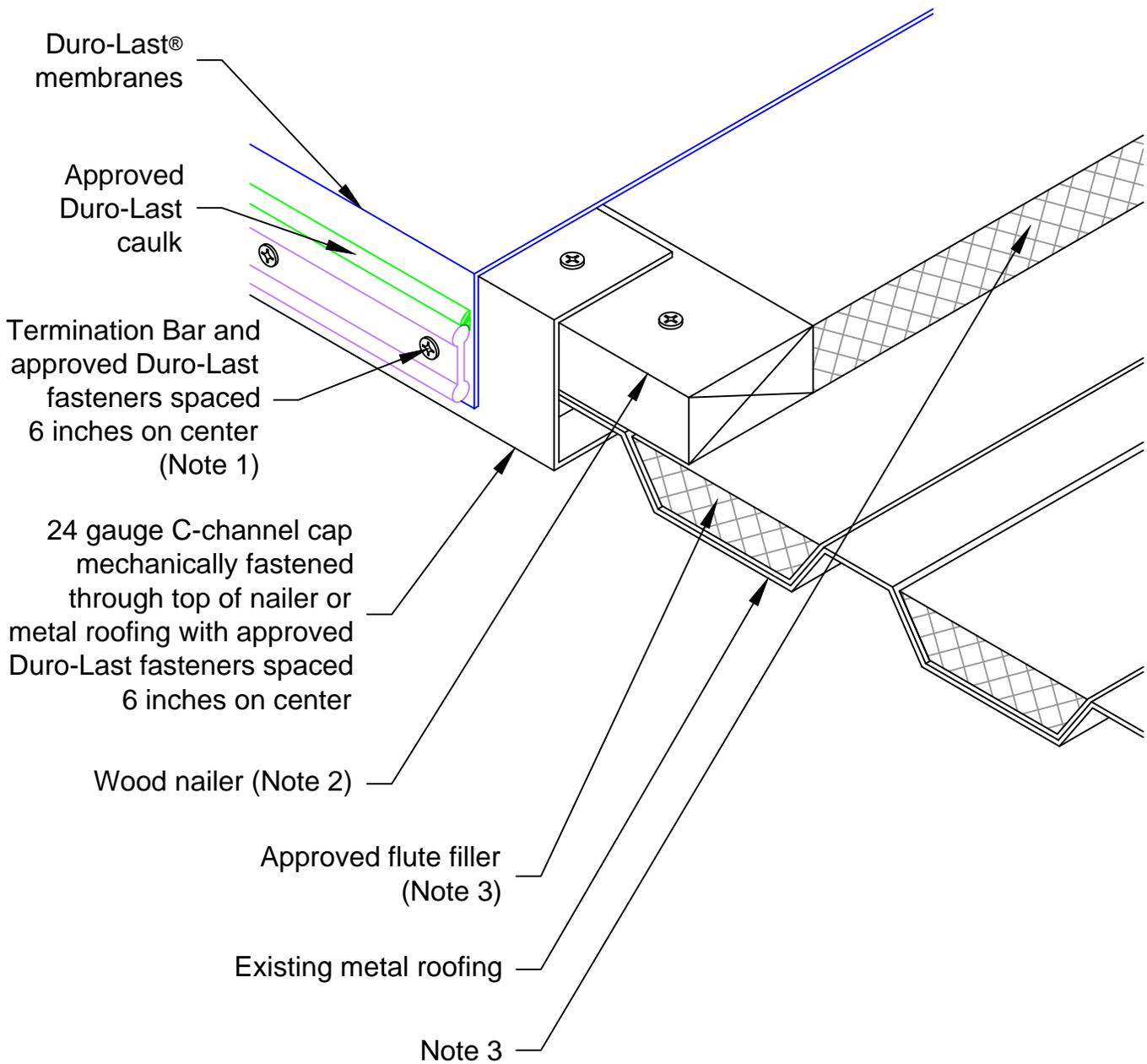
Note 1: Approved edge details may be used in place of Termination Bar.
