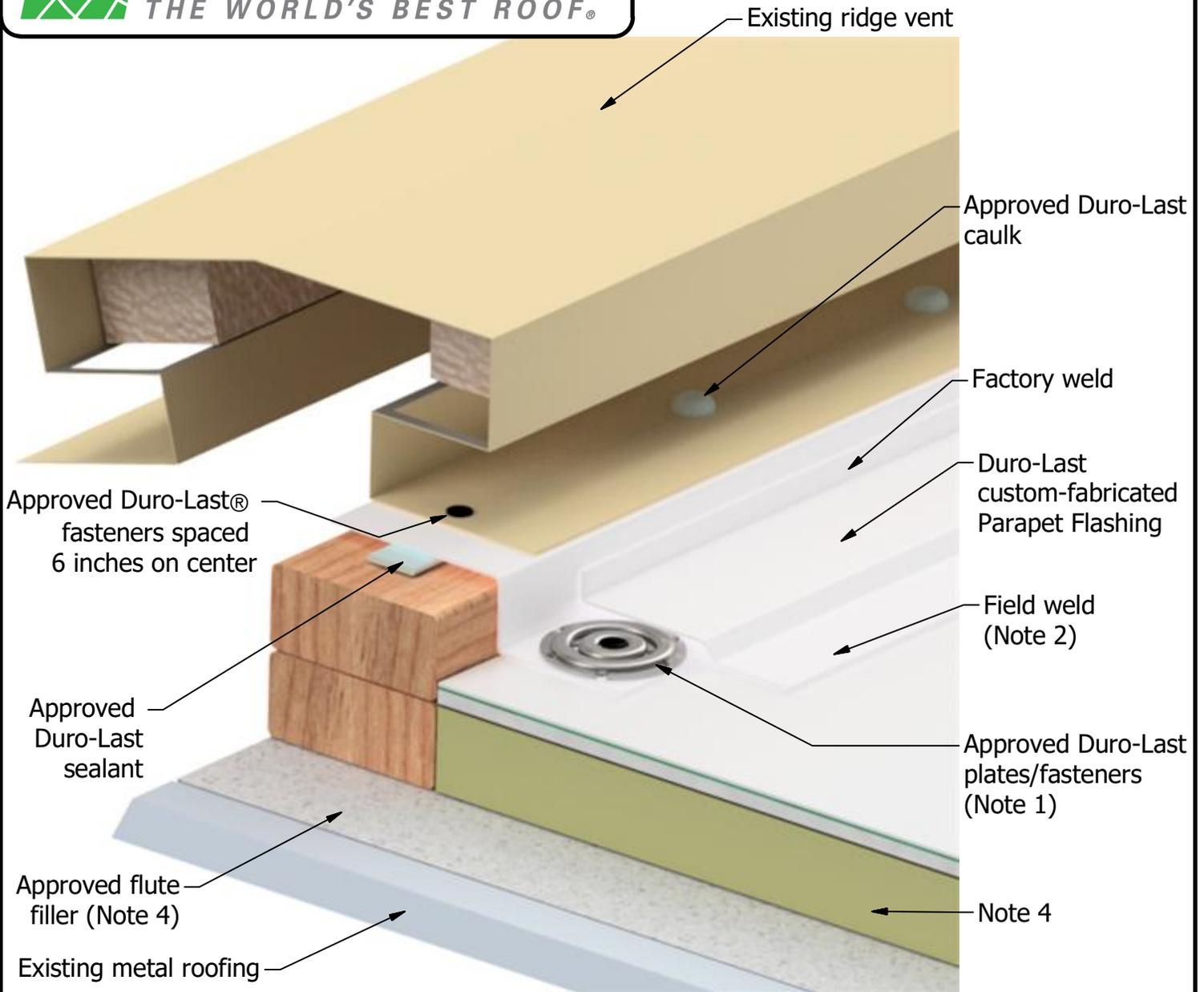
Note 1: Membrane fastening at deck-to-wall transitions and walls shall be same as per respective zones that area is located within (field, perimeter, corner).
