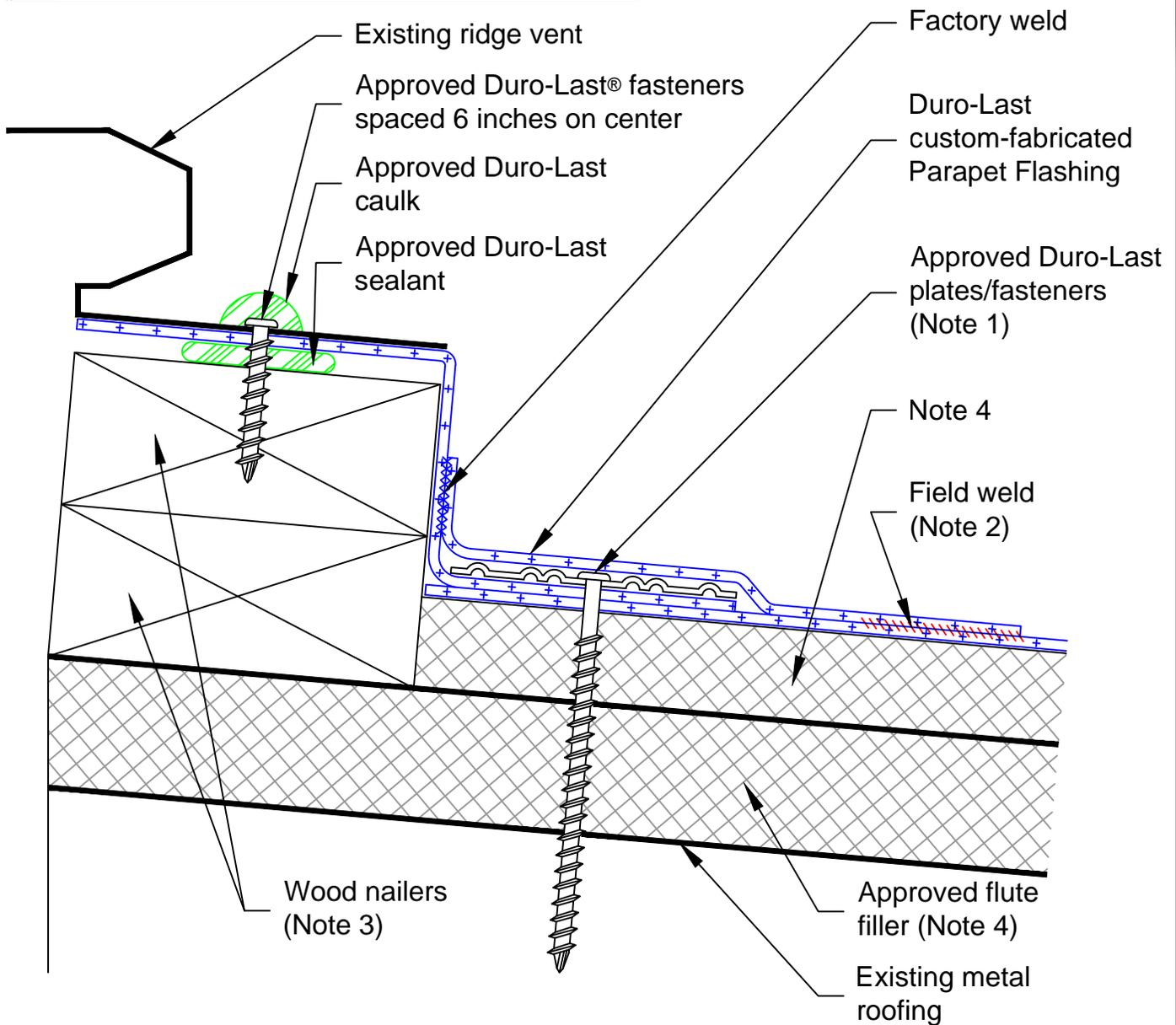
Note 1: Membrane fastening at deck-to-wall transitions and walls shall be same as per respective zones that area is located within (field, perimeter, corner).
