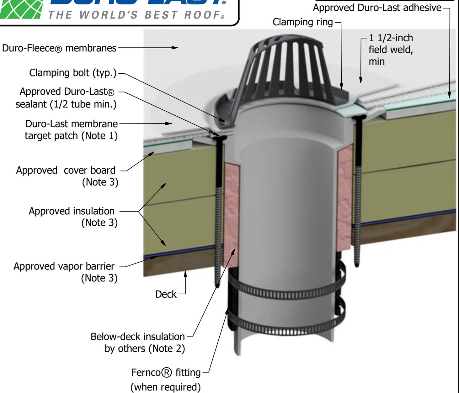
Note 1: Target patch must extend beyond drain sump to eliminate any hot-air welding within sump. If no sump is present, target patch must extend beyond drain assembly a minimum of 12 inches in all directions. Target patch must be same mil thickness as Duro-Fleece membrane.
