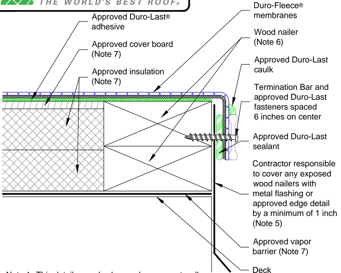
Note 1: This detail may also be used on parapet walls.
