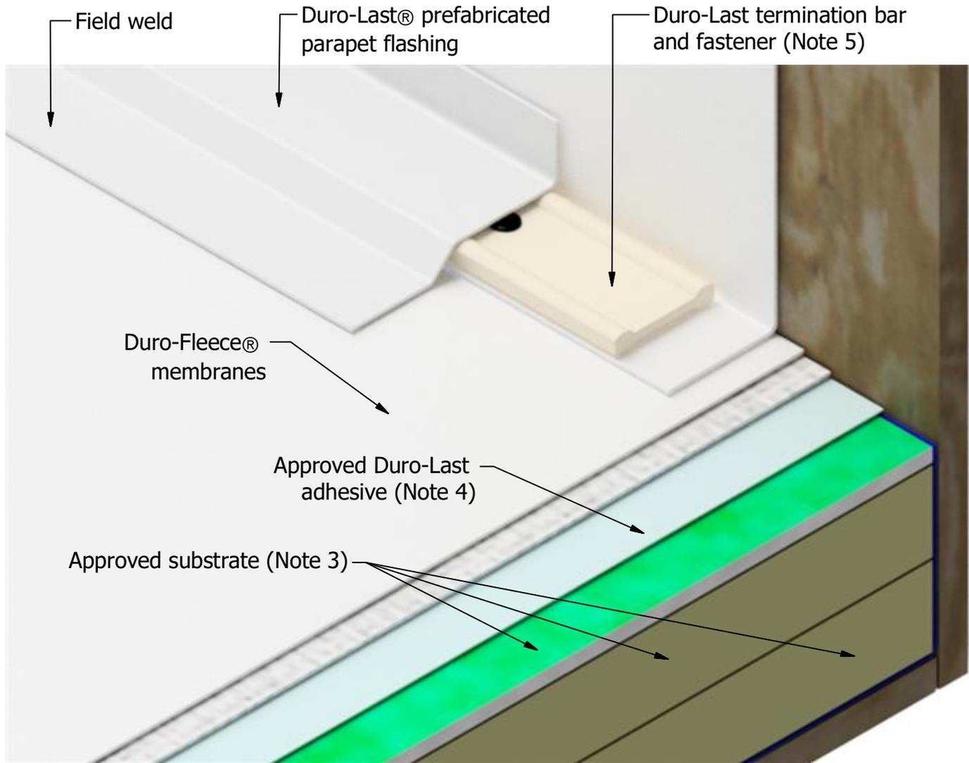
Note 1: Use one of these options for fastening the roof system at the roof-to-wall transition when the wall flashing is mechanically fastened. See DF6010 for adhering wall flashing.
