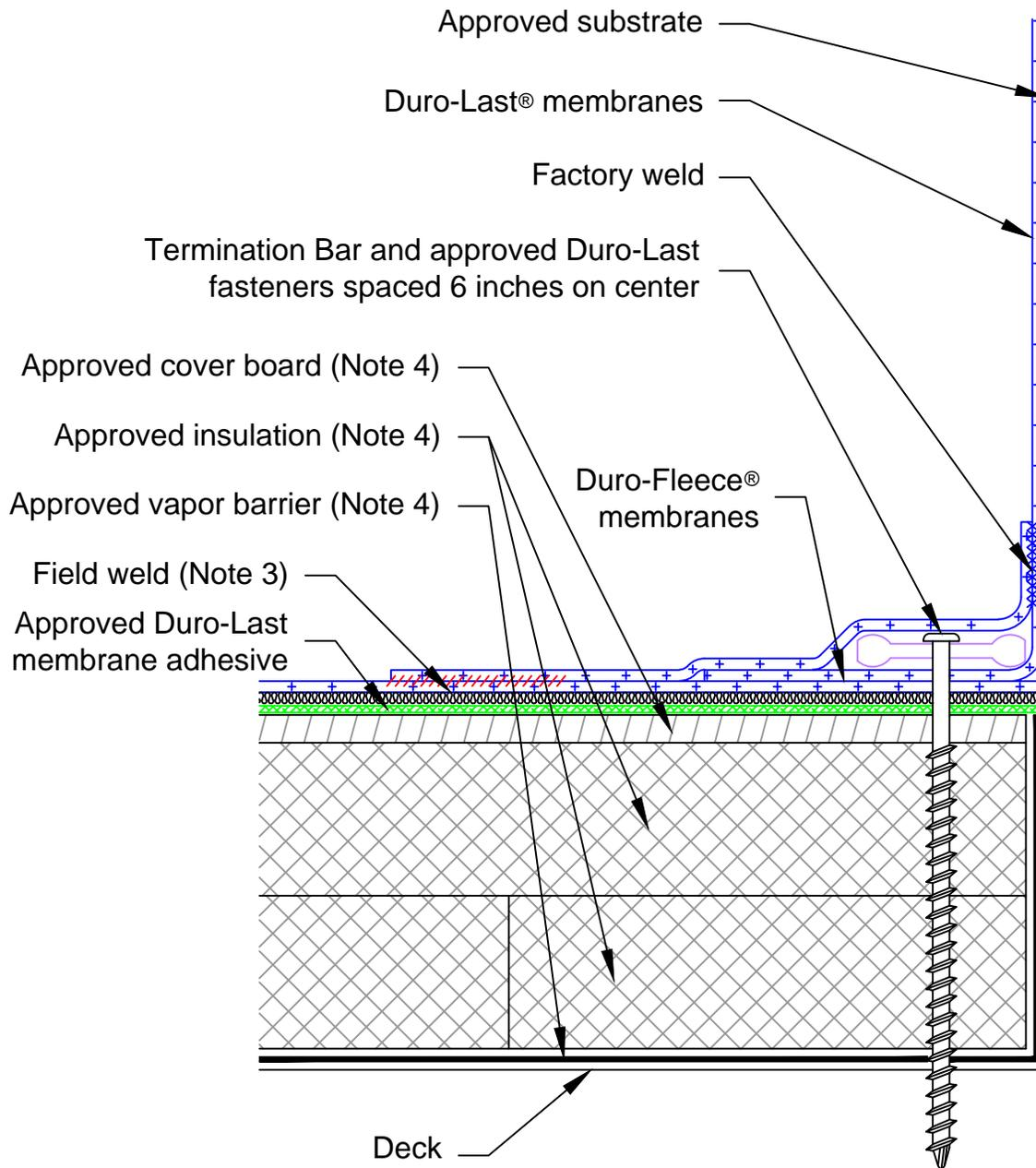
Note 1: When deck and wall membranes are adhered, refer to Detail Drawings DF6010 and DF6011.
