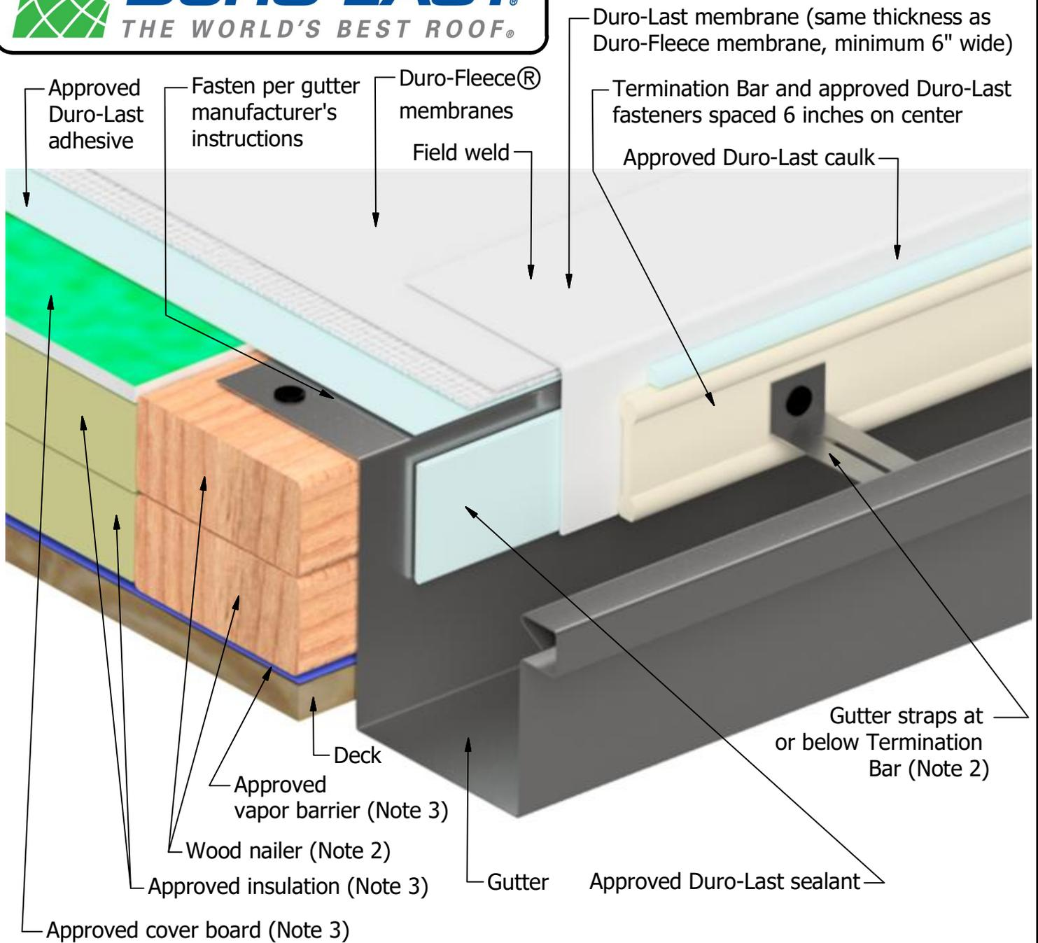
Note 1: A 1/4-inch gap is required between sections of Duro-Last termination bar.
