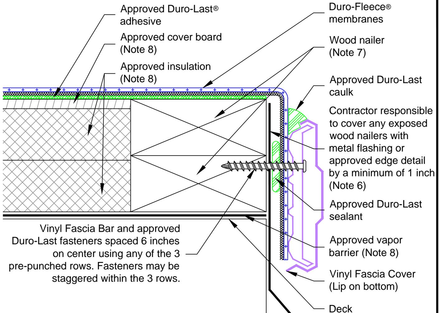
Vinyl Fascia Bar and approved Duro-Last fasteners spaced 6 inches on center using any of the 3 pre-punched rows. Fasteners may be staggered within the 3 rows.
