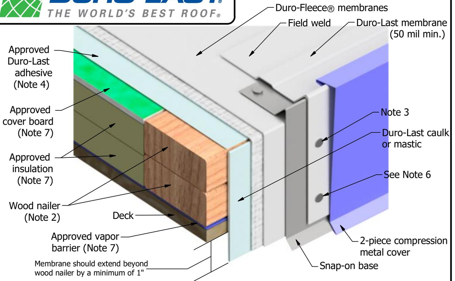
Note 1: This detail is not allowed when roof slope exceeds 2 inches vertically per 12 inches horizontally.
