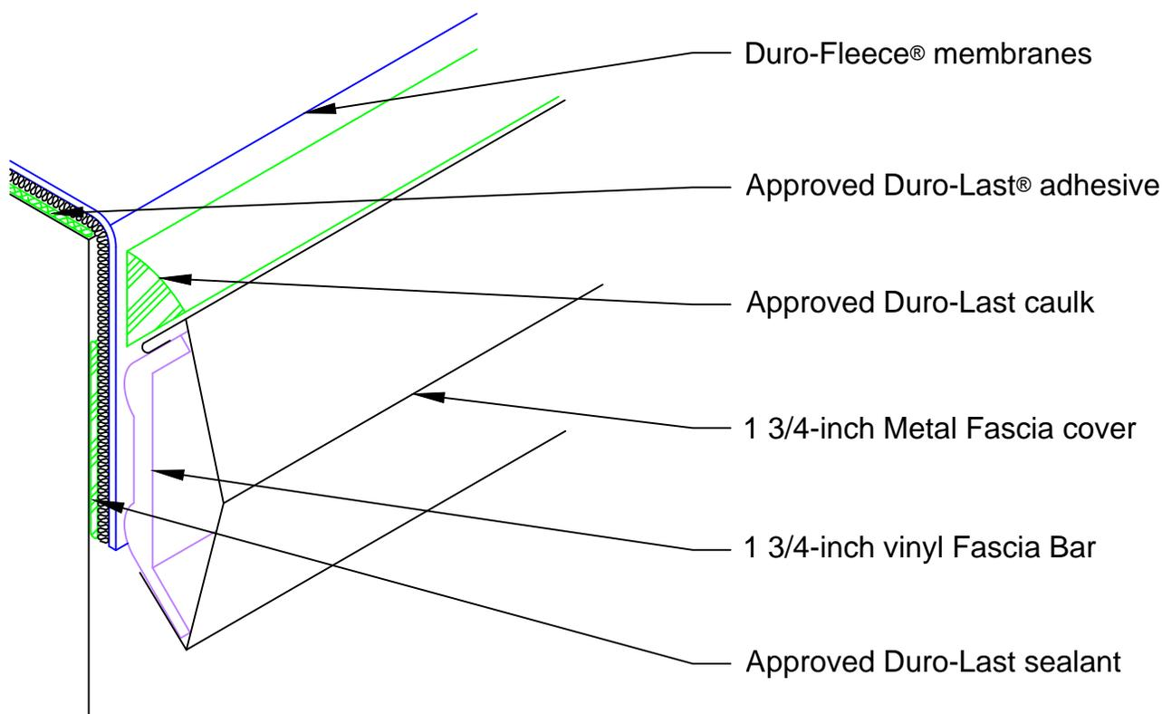
Note 1: This detail may also be used on parapet walls.
