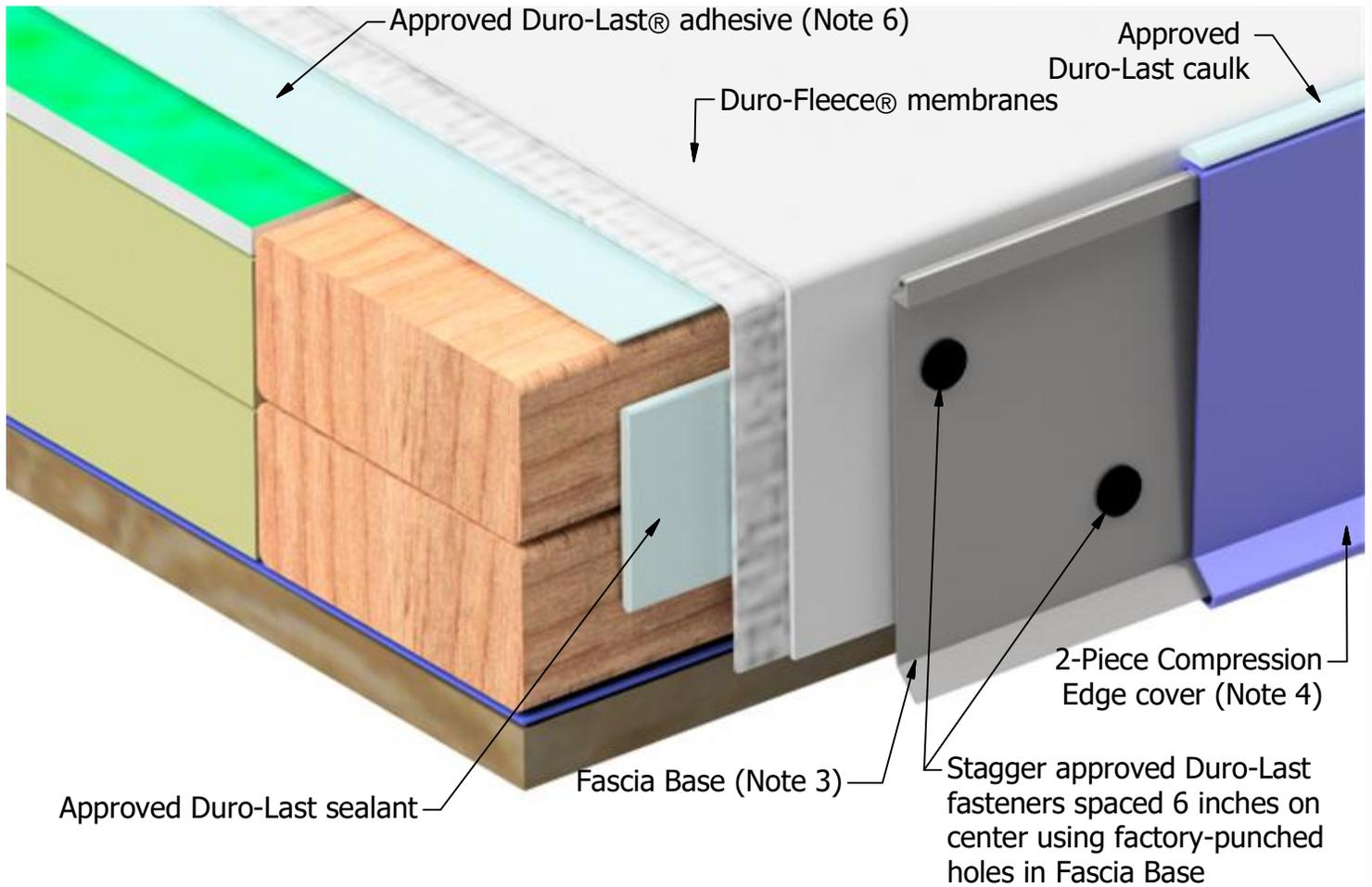
Note 1: A 1/4-inch gap is required between sections of duro-Last fascia base. Joints on the fascia base must be offset by a minimum of 12-inches from the joints in the metal cover.
