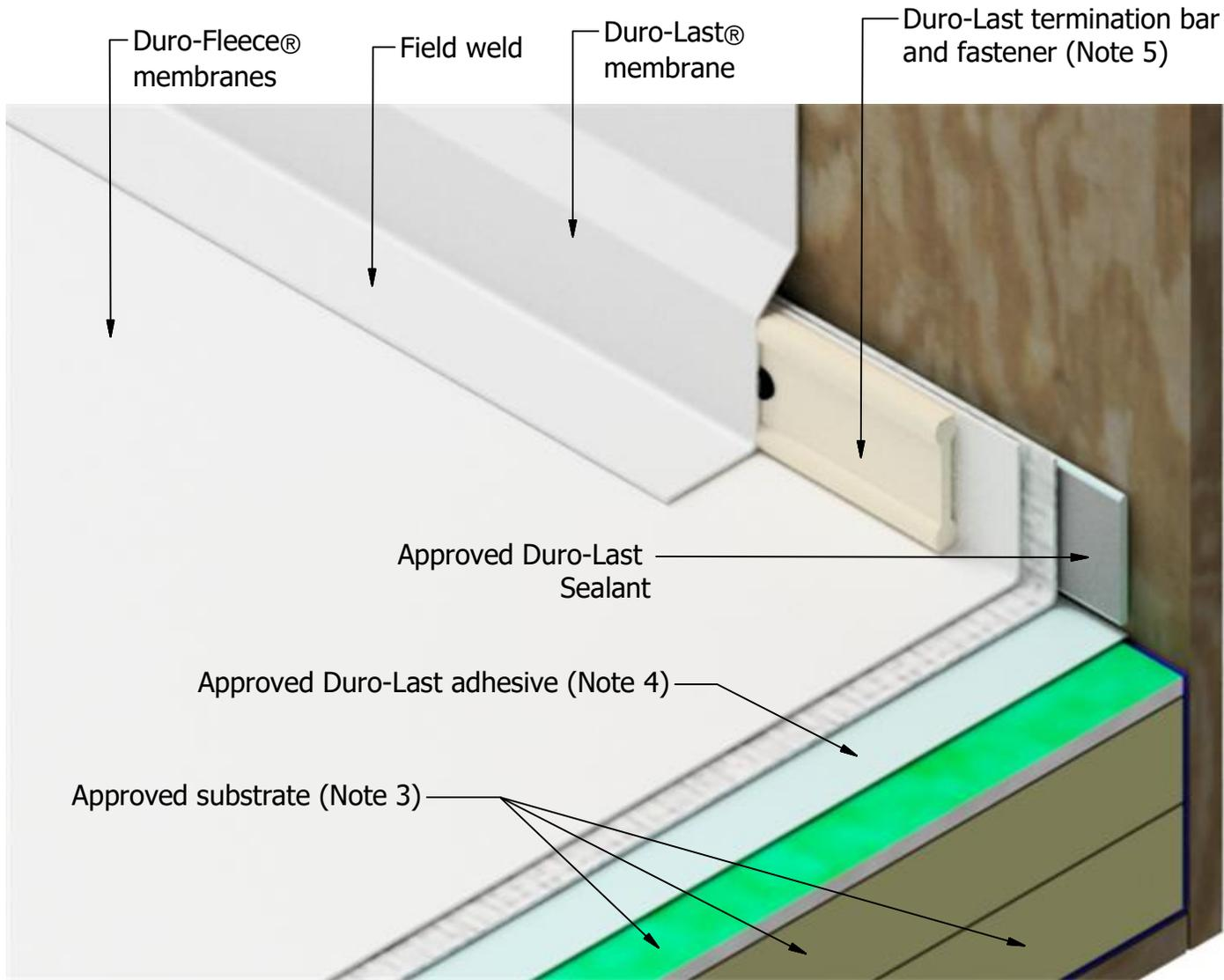
Note 1: Use one of these options for fastening the roof system at the roof-to-wall transition when the wall flashing is mechanically fastened. See DF6010 for adhering wall flashing.
