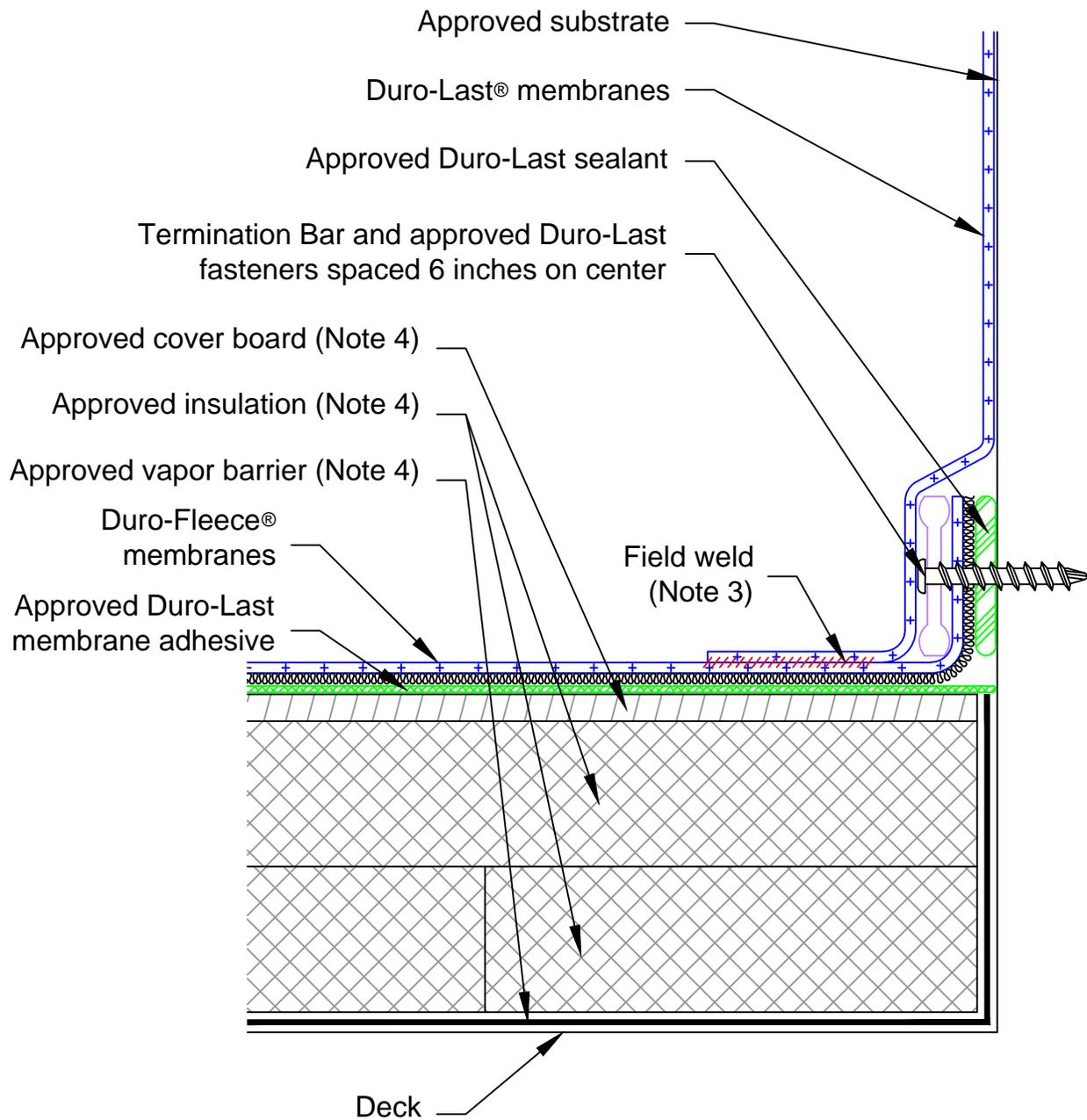
Note 1: When deck and wall membranes are adhered, refer to Detail Drawings DF6010 and DF6011.
