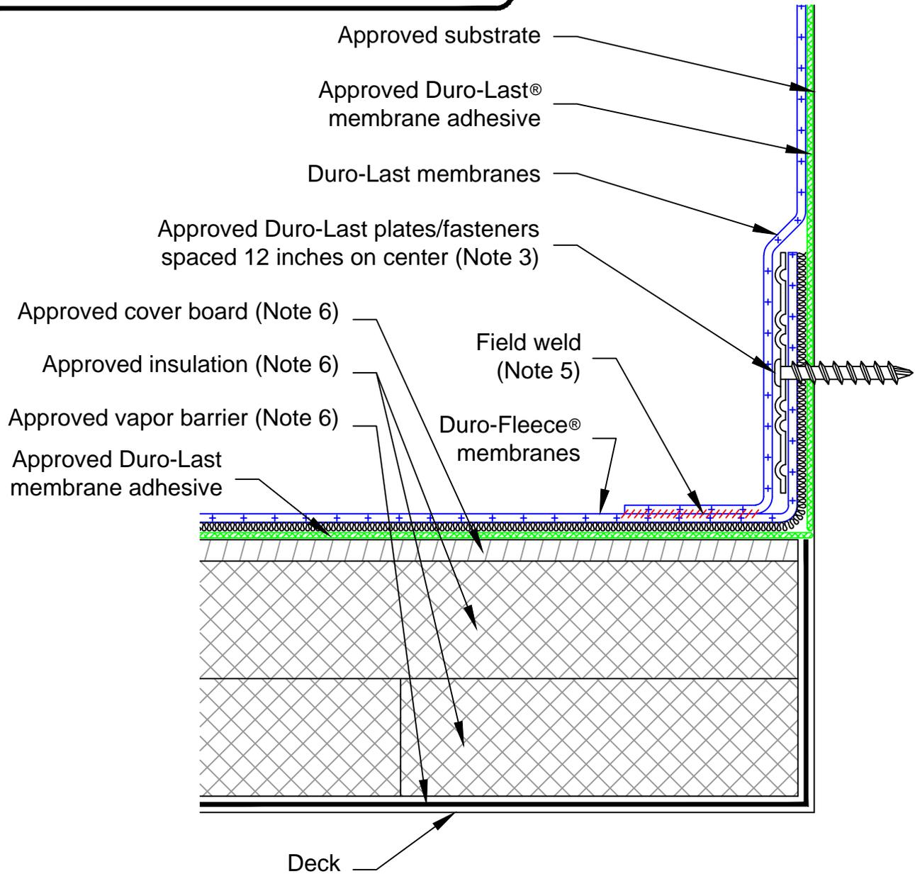
Note 1: When deck membrane is adhered and wall membrane is mechanically fastened, refer to Detail Drawings DF6000 and DF6001.
