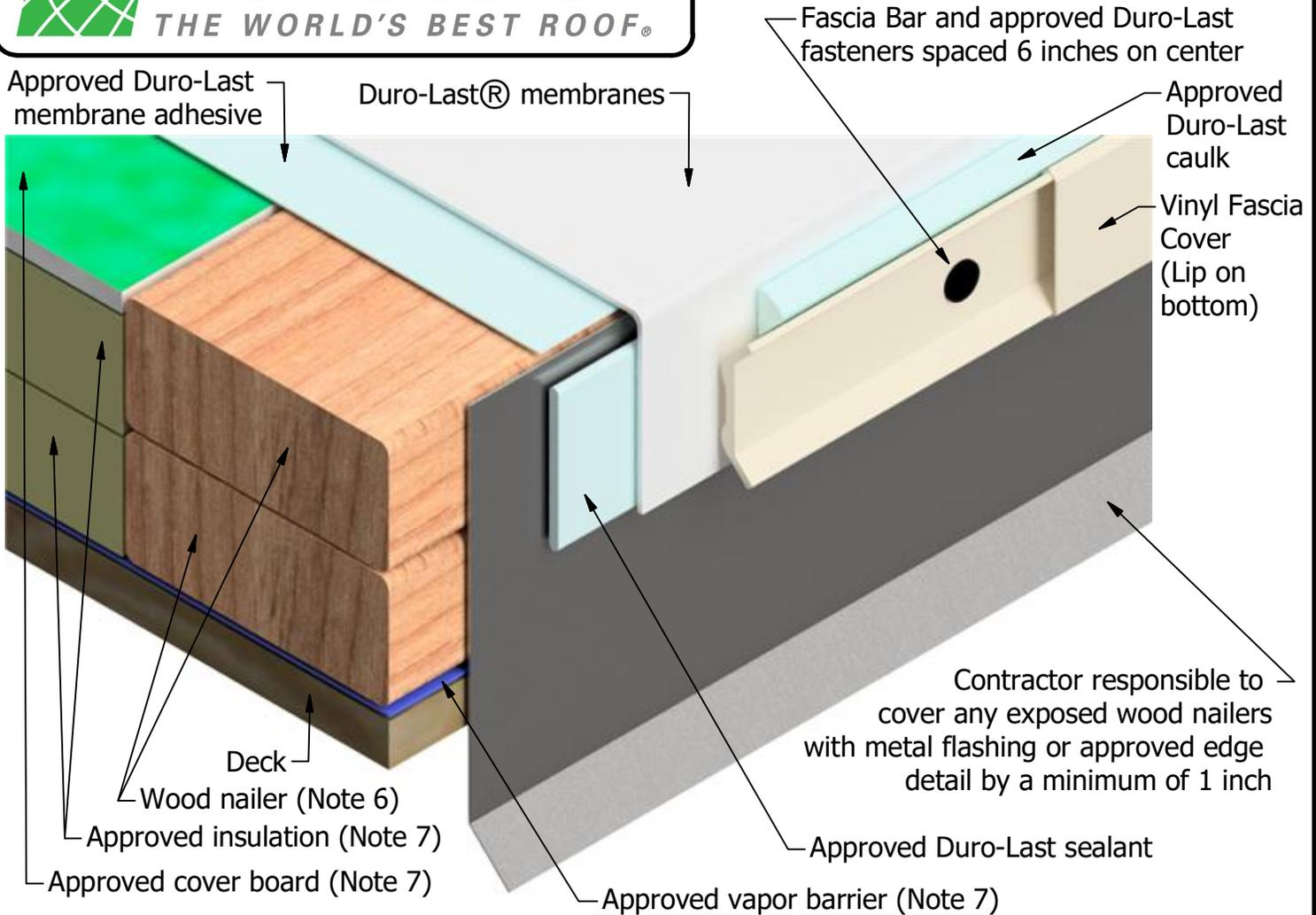
Note 1: This detail may also be used on parapet walls.
