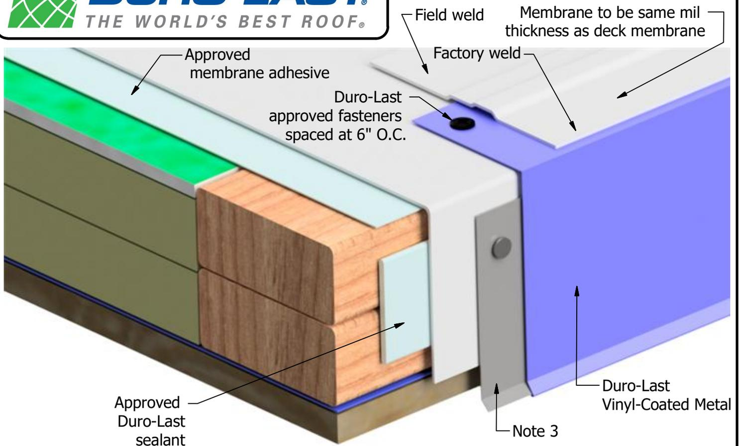
Note 1: An overlap of 1 1/2-inches will be required between sections of vinyl-coated metal. A bead of caulk is required in each overlap.
