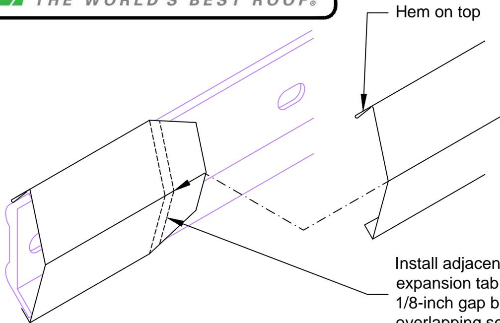
Install adjacent edging over expansion tab and allow for 1/8-inch gap between overlapping sections
