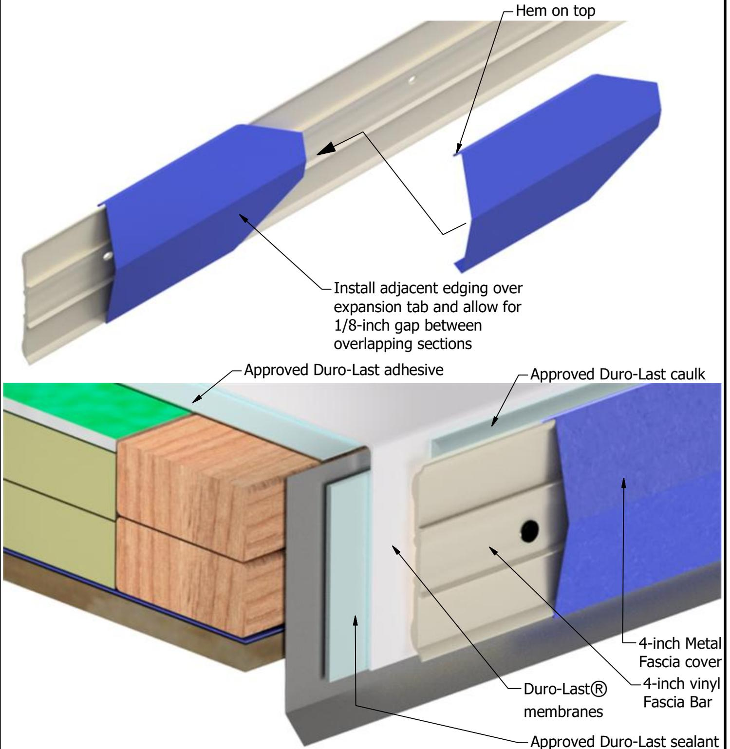
Note 1: This detail may also be used on parapet walls.
