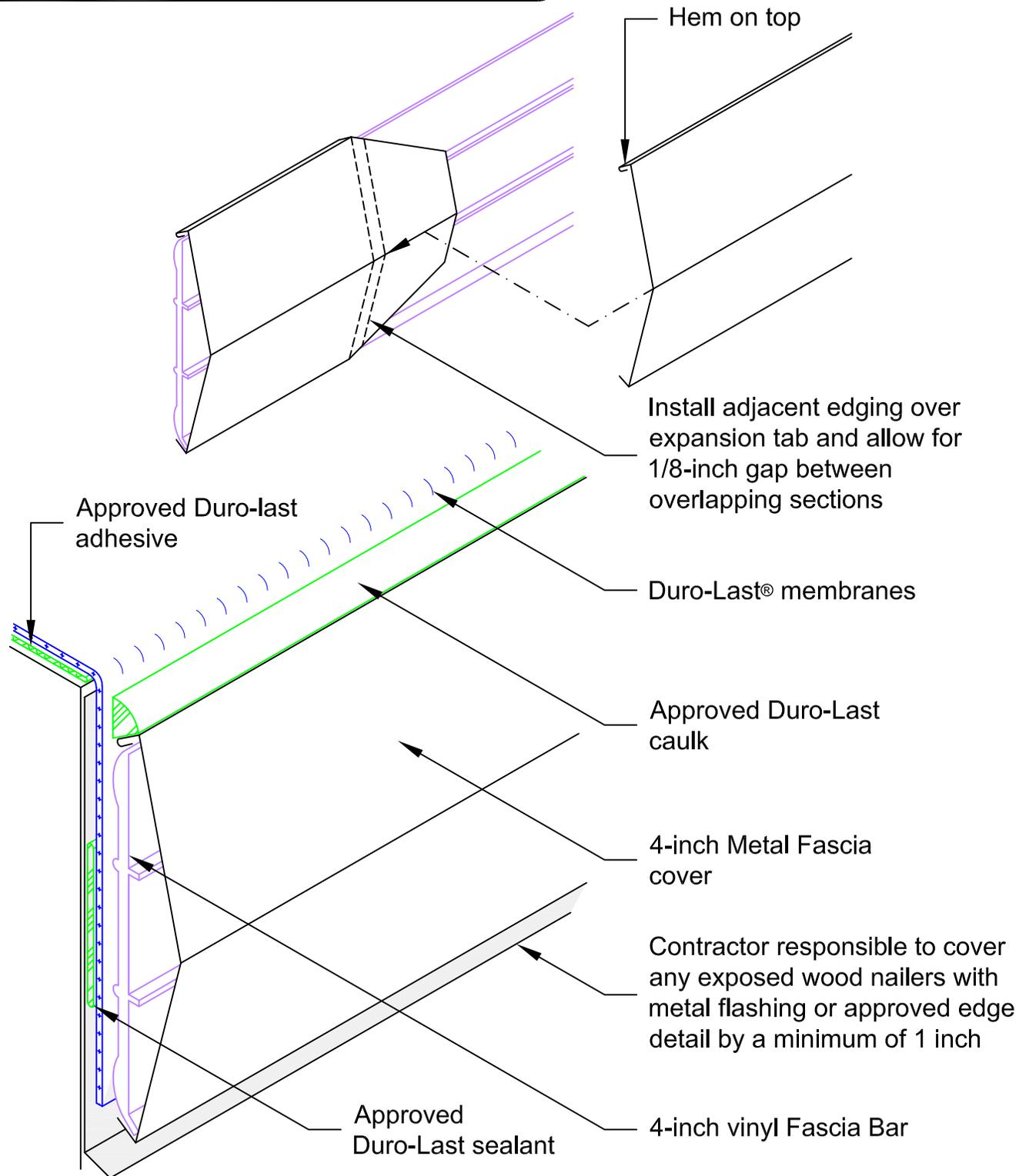
Note 1: This detail may also be used on parapet walls.
