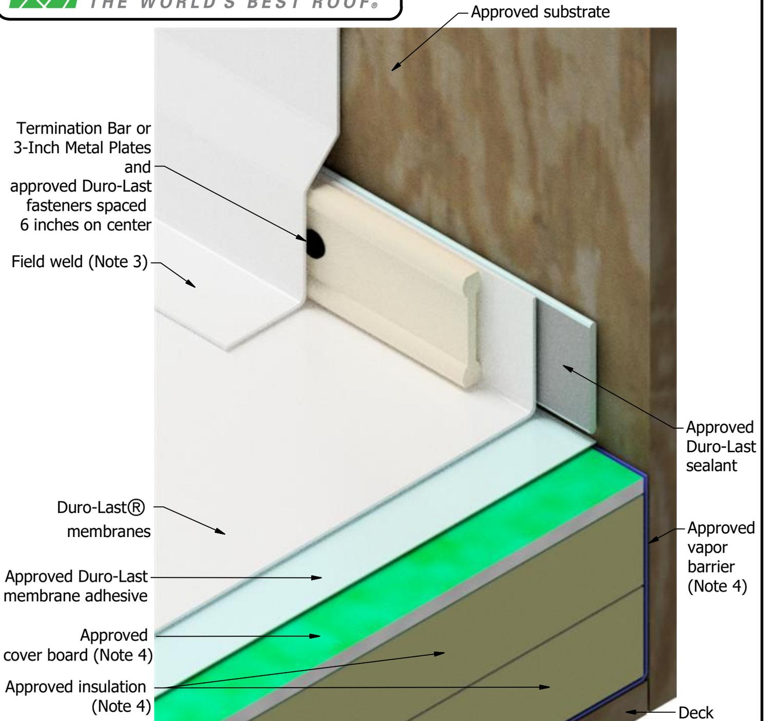
Note 1: When deck and wall membranes are adhered, refer to Detail Drawings AS6010 and AS6011.
