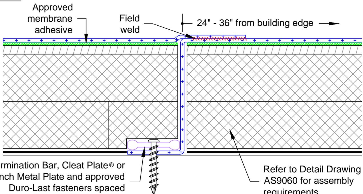
Termination Bar, Cleat Plate® or 3-Inch Metal Plate and approved Duro-Last fasteners spaced 6 inches on center
