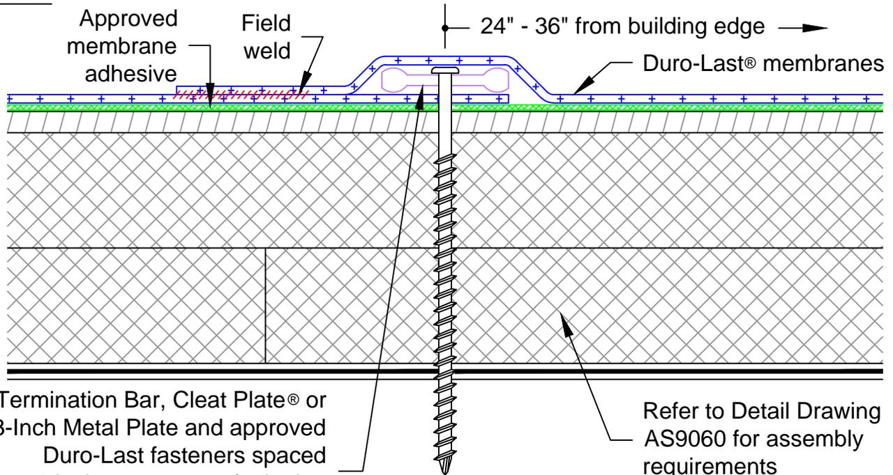
Termination Bar, Cleat Plate® or 3-Inch Metal Plate and approved Duro-Last fasteners spaced 6 inches on center (stripping may also be welded to both sides of peel stop row)
