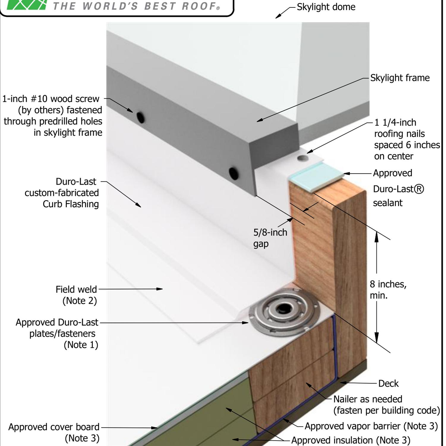
Note 1: Deck membrane shall be fastened around perimeter of roof penetration as per respective zone the skylight is located within (field, perimeter, corner).
