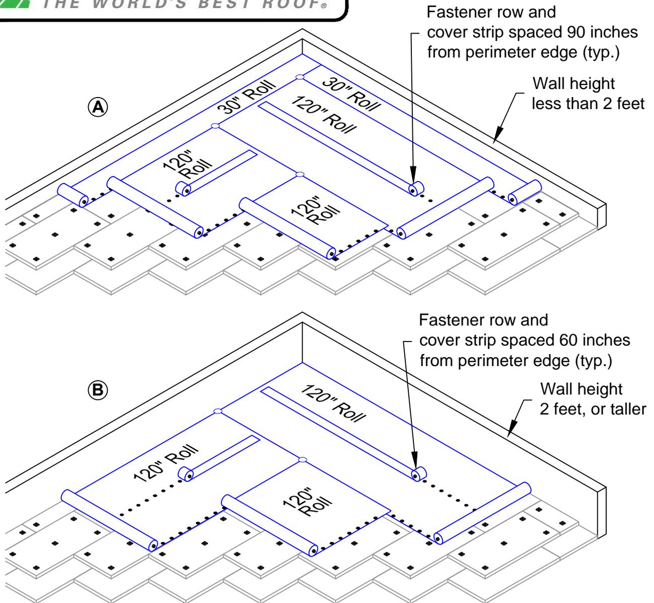
Note 1: Cover strips shall be wide enough to accommodate a 1-1/2-inch wide weld on all sides. Stripping can be made of either DT or DL membrane of any thickness. DL EV stripping shall only be used on DL EV membranes.
