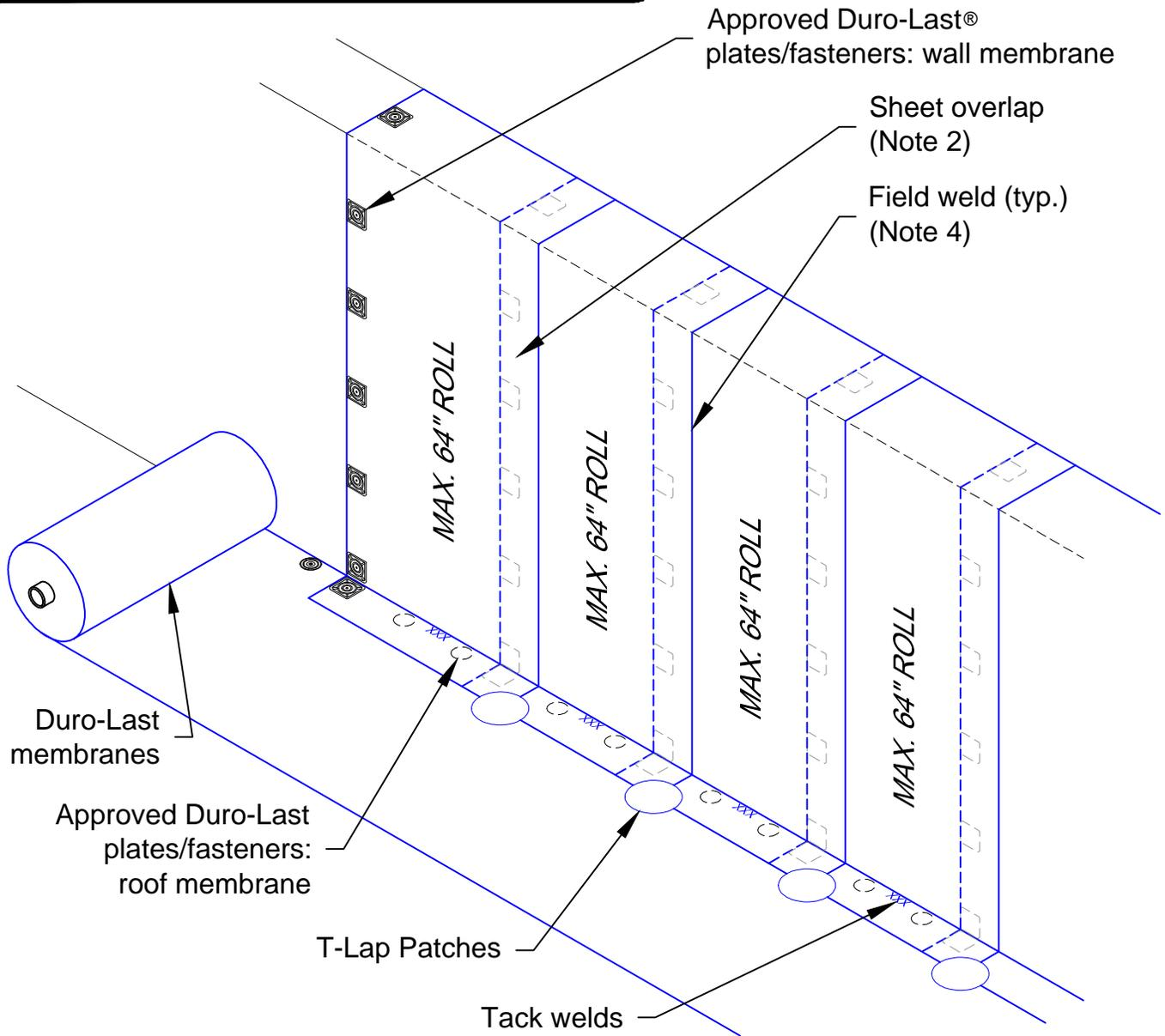
Note 1: Refer to the *Roll Good Mechanically Fastened Roofing System* specification for the fastener spacing requirements on the wall and roof deck. Fastener spacing for wall membrane will be same as perimeter and corner fastening requirements for deck membrane.
