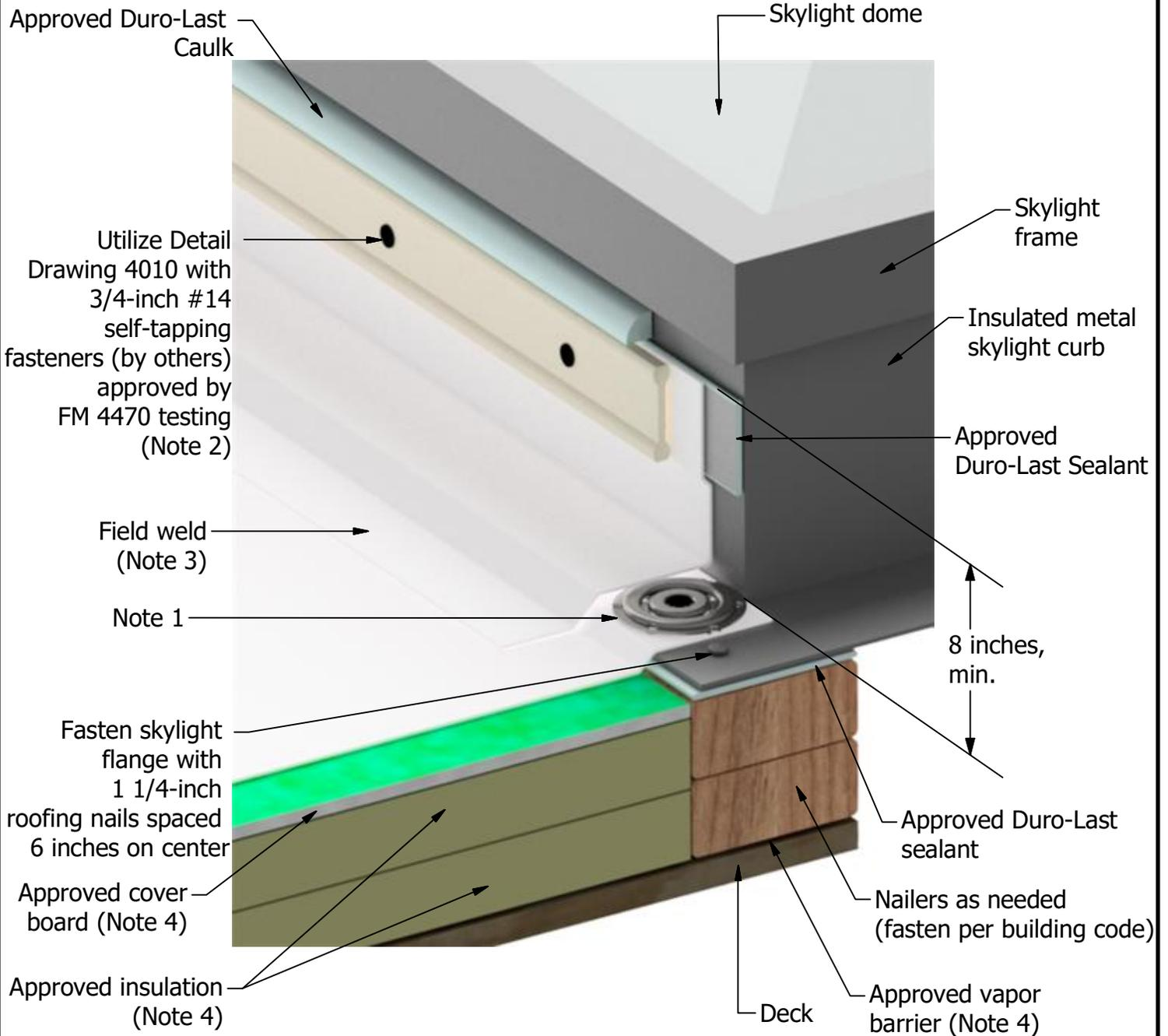
Note 1: Deck membrane shall be fastened around perimeter of roof penetration as per respective zone the skylight is located within (field, perimeter, corner).
